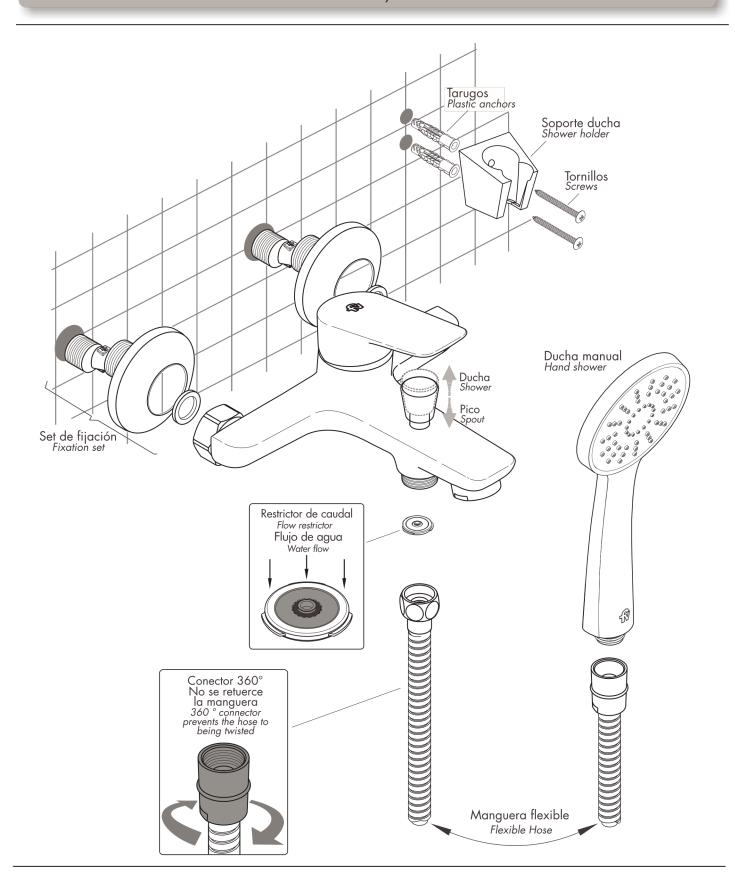
**Z310/M1** Juego monocomando exterior pared, para ducha y bañera, con transferencia y ducha manual incluída. Single handle shower/bath wall mount mixer, with eccentric couplings, diverter valve, with hand shower included.
